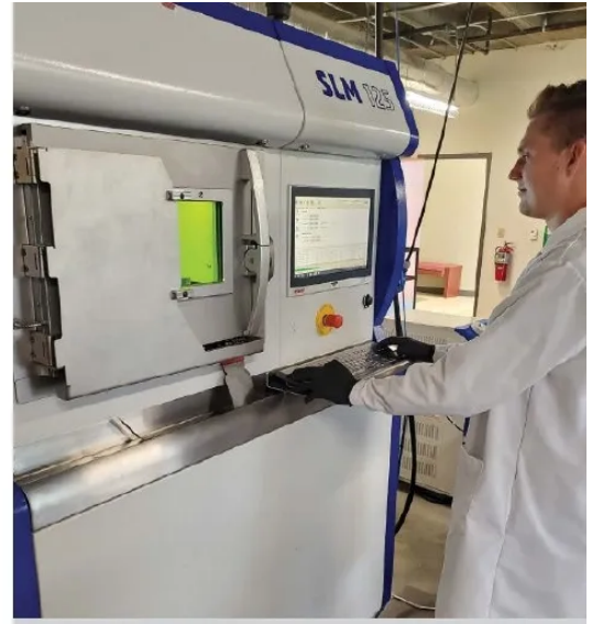
(Above) Former research students of Dr. Jackson using a 3D metal printer and (below) tensile testing the materials printed to determine their strength.
