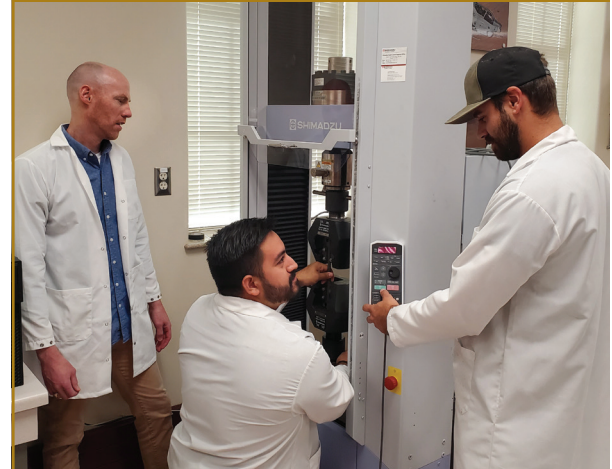
(Top) Former research students of Dr. Jackson using a 3D metal printer and (bottom) tensile testing the materials printed to determine their strength
